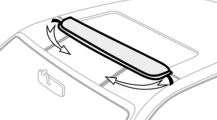
After positioning the sunroof deflector, remove the masking tape and carefully remove the remaining protective liner by pulling on the loose ends. Do not break the protective liner.
