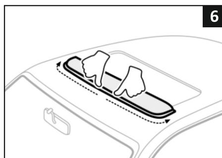
Press down firmly on the deflector at the bonding points to ensure good adhesion.
