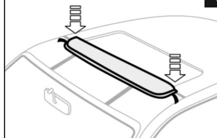
Place the sunroof deflector aligning with the previously marked locations. Press lightly on the exposed areas of the adhesive tape and check the position of the hatch.
